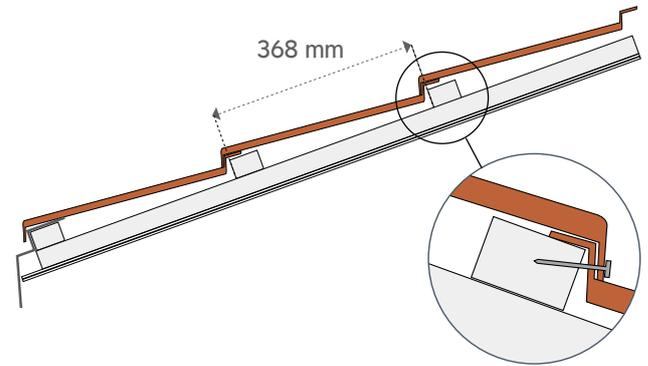
The panels are placed onto battens spacing 368 mm. The downturned front edge and the upturned rear edge of each tile provides a strong, weatherproof, overlapping and interlocking roof covering. Each panel is secured by 4 nails in the front downturned edge into the side of the batten, positioned out of the water course.
